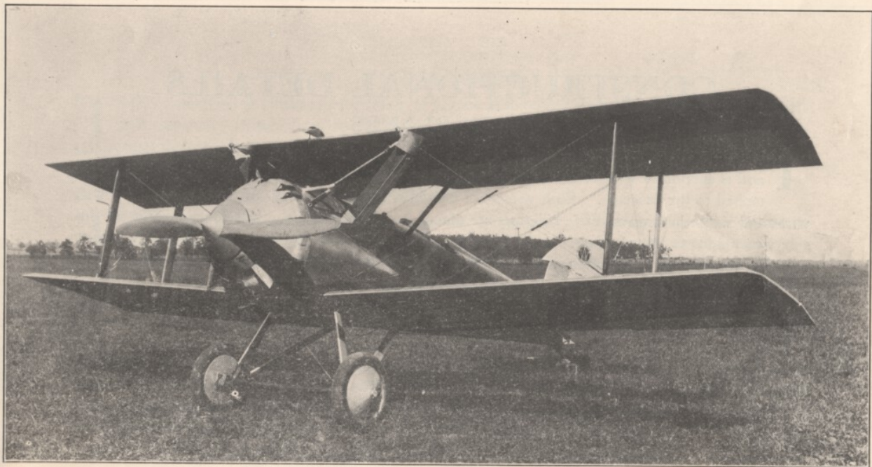
This plane has a safety factor of 8 throughout and will withstand the roughest treatment, insuring safety.
